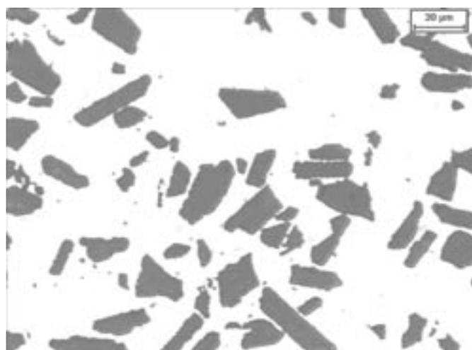
Fig.2. Microestructura del material A6061MMC.
